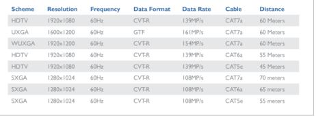
Distances are achieved using single lengths of trunk/bulk cable. For each break/patch connection reduce distance by 5 meters. For resolutions/ data rates of less than 1280x1024 /108MP/s, add 10 meters. Preferably patch cables should be of type CAT7a and less than 2 meters. Patch cables over 2 meters must be CAT7a.
